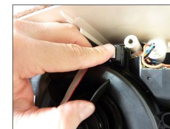
3. Mount the fixing cover, included in the scope of delivery, at the top right with the respective fillister head screw.
