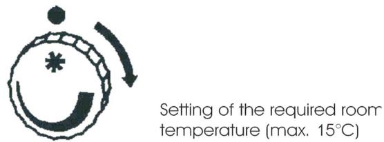
To set the required room temperature: turn the knob to the right as far as it will go and wait until the required temperature has been reached. Turn the knob then slowly back again until the control lamp has been extinguished. The position of the knob now corresponds to the required temperature. After reaching the room temperature of max. 15°C the heater switches off automatically.
